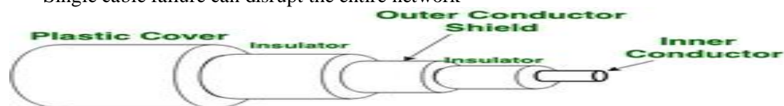
Figure of Coaxial Cable
